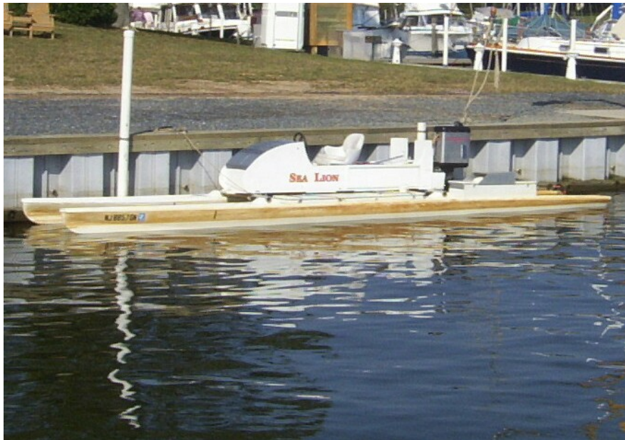
Paul Kydd's Electric Boat Using Lithium Ion Batteries (160 lbs vs 720 lbs of lead acid) Notice water line is significantly above water Lawrenceville, NJ Yes – he won first place in an Oct 1 Race!
