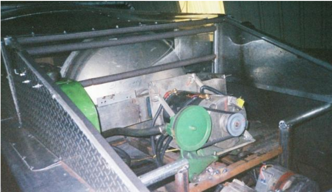
The vehicle is driven by the flywheel operated at a constant 4500 rpm. The tail shaft of the FBI-4001A motor drives the hydraulic control system.
