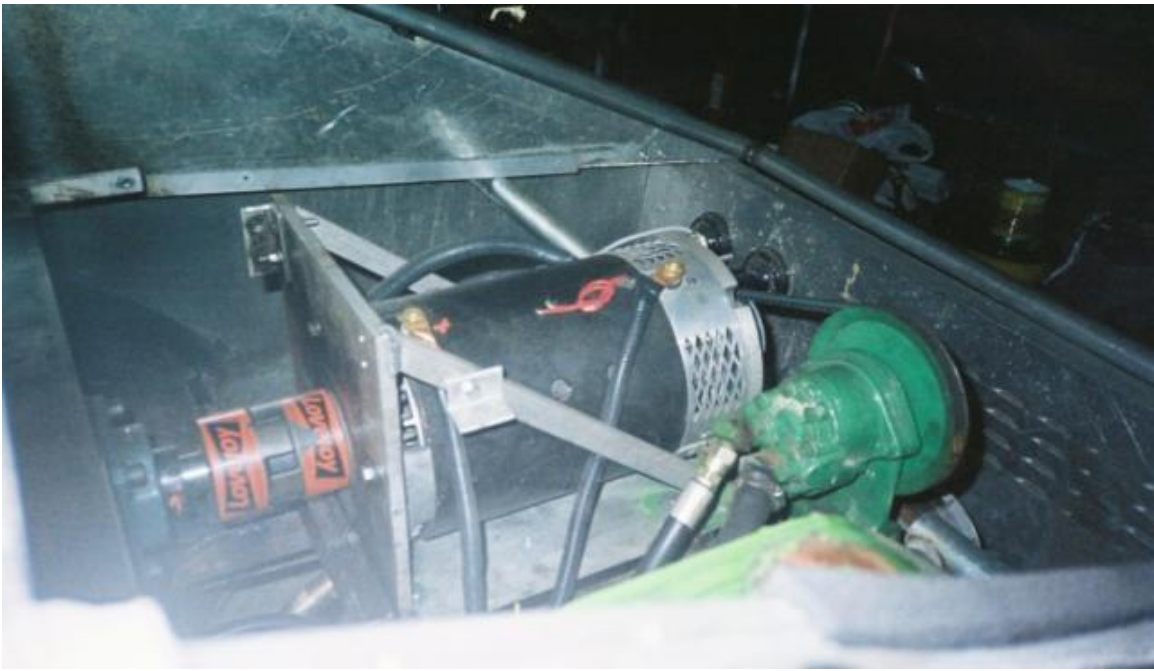
The Lovejoy Coupling is driving the flywheel; The tailshaft is driving the hydraulics for acceleration and deceleration.
