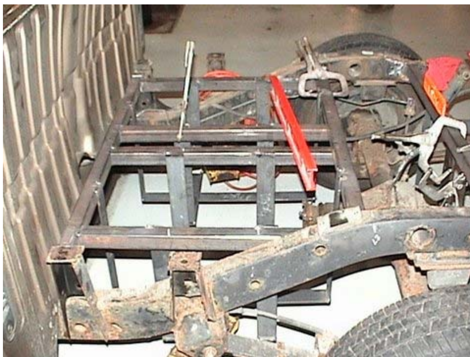
The Isuzu has limited space forward of the Rear axle for the battery boxes.
