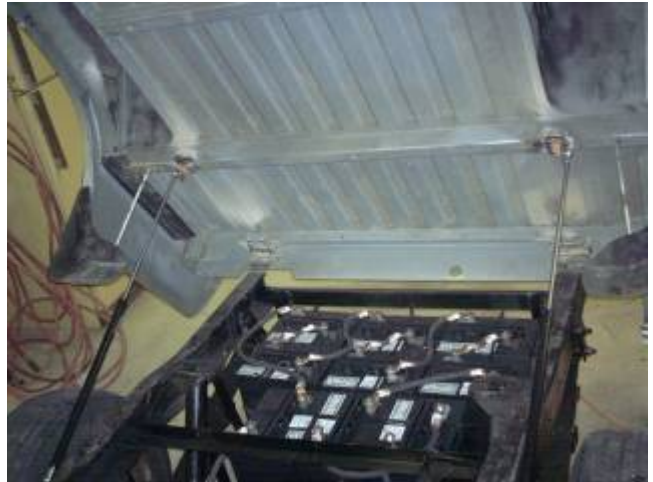
With our new 200lb lifts and 15 inch stroke This bed allows easy access.
